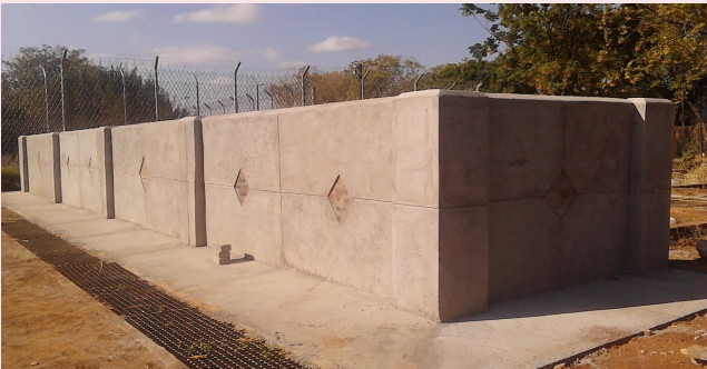
Manufactured Sand Experimental wall
