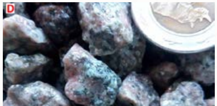
Figure 18: Coarse to medium grained found both in the eastern and southern Botswana, the material qualify for road and building construction. Further crushing of these rocks, using cone crushers produces manufactured sand, which is suitable for construction buildings.
