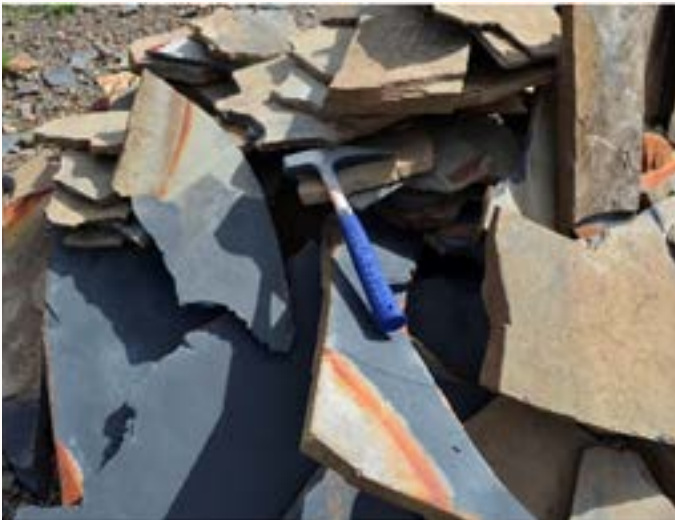
Figure 17: Dipotsana slate is grey in colour when it is fresh, but it weathers reddish-brown depending on the period it took in contact with the fluids which results in oxidation of the top most surface of the slate.
