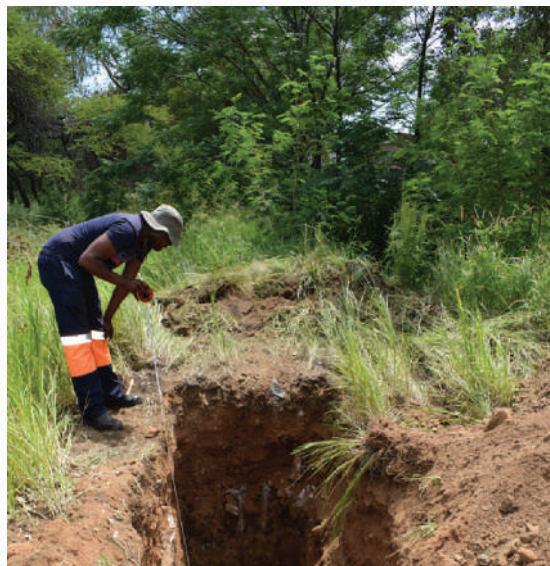
Picture: Groundwater level measurements (Piezometric surface / water-table) intersected between 2.3 and 2.8 metres
