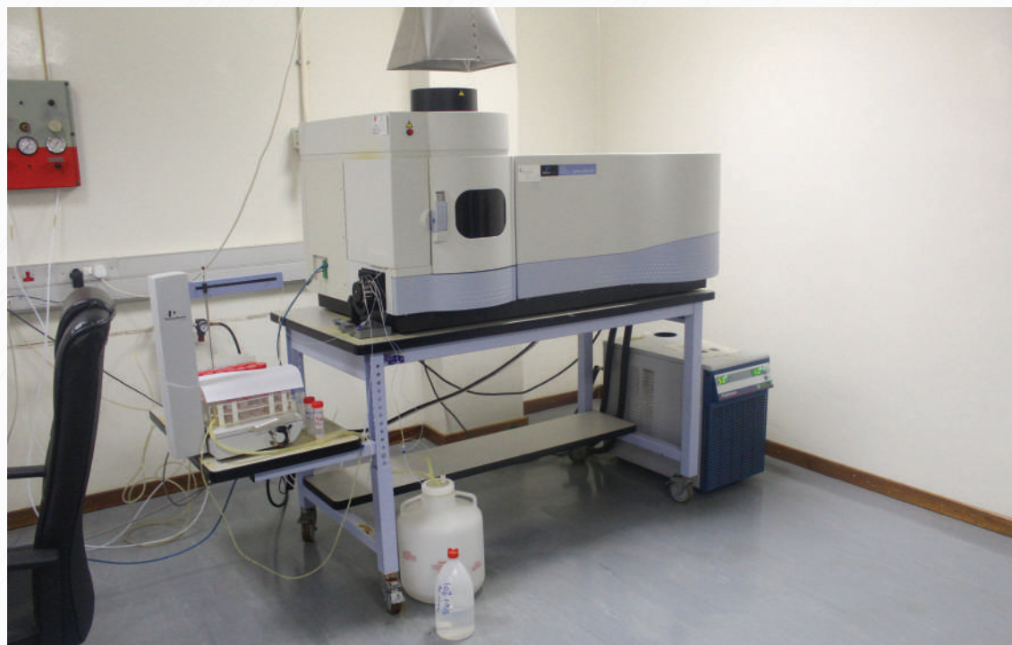
Picture: Optical Emission Spectrometer (ICP - OES 7300 DV)
