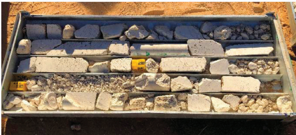
Figure 6: Downhole core of the Letlhakeng Boreholes.
