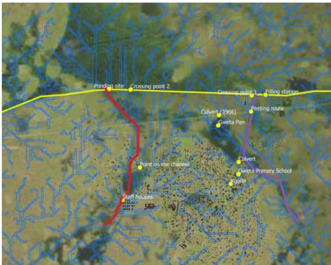
Figure 15: Proposed short-term solutions for Gweta (red and violet polyline) using storm water drainage to carry flooding water from A3 road. The blue lines are the natural drainage network delineated from DEM
